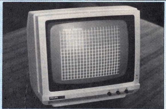
PHILIPS FILLIP — A 12in video monitor for personal computers, the TP 200, has been developed by Philips. Retailing at £75 the monitor offers an anti-glare screen giving clear definition with 80-25 character resolution. It has been designed for use with most micros, including the BBC and the Apple II. The unit has an extendable stand fitting which allows you to tilt the screen to the required angle. It is distributed by EMCO (01-737 3333) in London and Vako Displays (061-652 5111) in Oldham.
